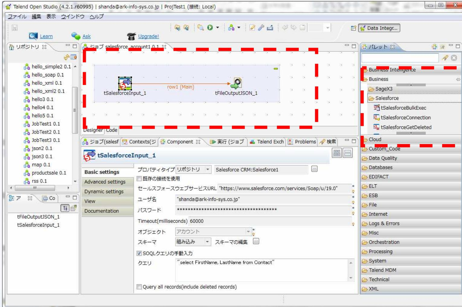
The screenshot displays the Talend Open Studio (4.2.1.r60995) interface. The main workspace shows a job named 'salesforce\_account1.0.1' with a flow from 'tSalesforceInput\_1' to 'tFileOutputJSON\_1'. The 'tSalesforceInput\_1' component is selected, and its configuration panel is visible on the right. The configuration includes:
